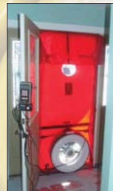
Photo of Blower door
